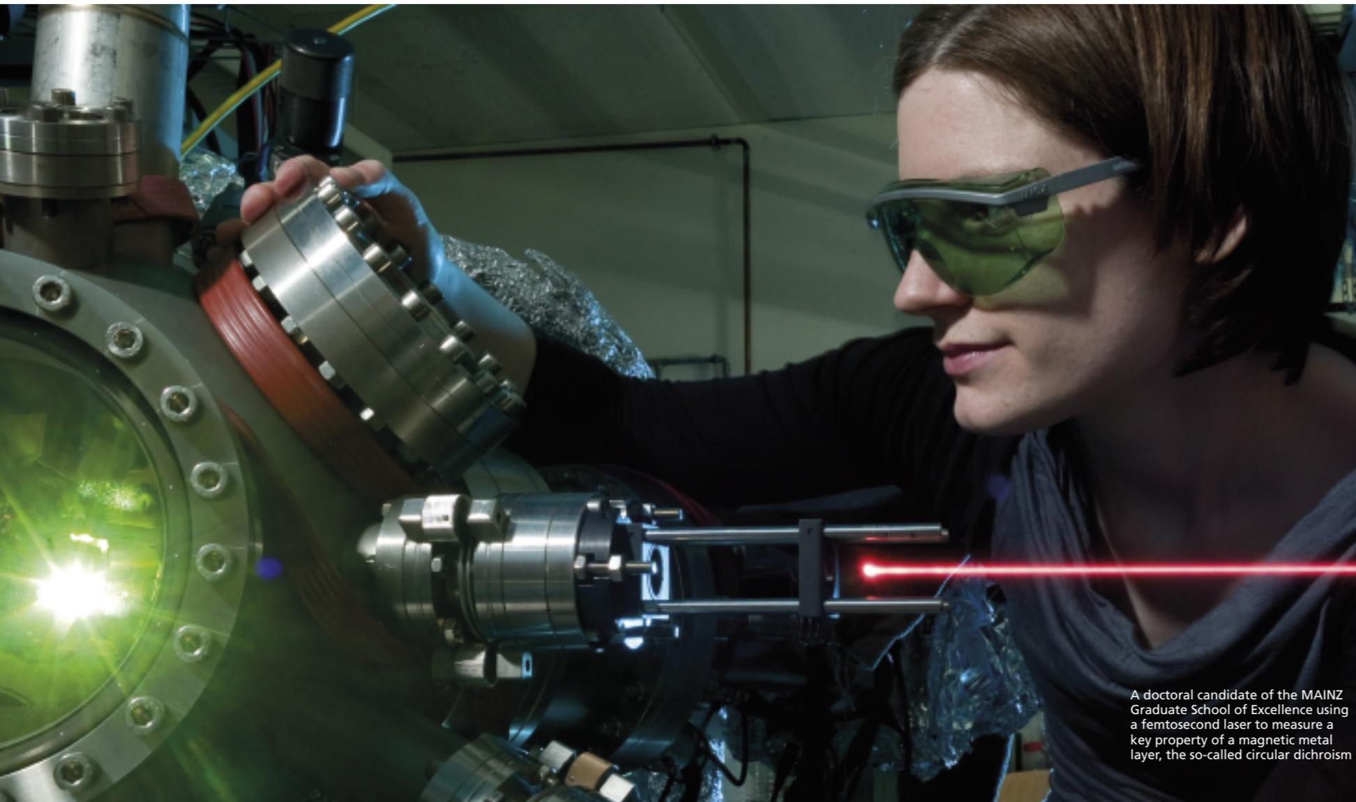
A doctoral candidate of the MAINZ Graduate School of Excellence using a femtosecond laser to measure a key property of a magnetic metal layer, the so-called circular dichroism
